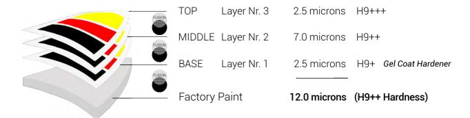
Trinity Fusion Ceramic Coating is based on silicon-nitrogen polymers and ceramics derived from reactions of dichlorosilane with ammonia. This chemical platform is more expensive but gives far much more durability and is a must to meet customer expectations / or to avoid customer complaints.
